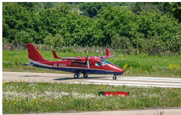
Figure 11 - Tecnam P2006T (MTOW 1230 kg, Max cruise speed 269 km/h) Min. Speed 115 km/h, 4 seats)
