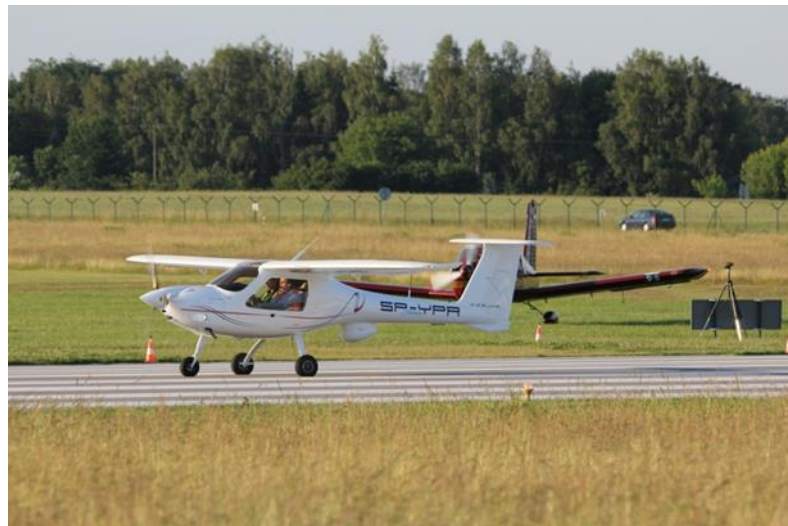
Figure 5 - Optionally Piloted Vehicle (MTOW 495kg, Max. Airspeed (Vne) 270 km/h Min. Speed 65 km/h 2 seats)
